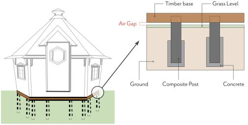
The composite posts attach to the timber base frame and penetrate the ground. The posts are individually encased in concrete to lock them into position and provide years of support.
