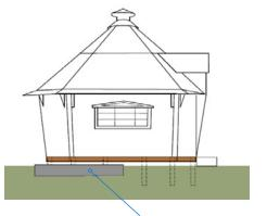
If you have an old concrete base or patio area that is covering part of the cabin location, we can often accommodate this with our base system. Some posts rest on the existing hardstanding, whilst the remainder are concreted into the ground as normal.
