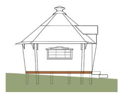
One advantage to our base system is that we can easily work with sloping ground without the need to excavate or flatten the ground itself. The base frame is levelled using the posts. Some steps and additional base cladding may be required.
