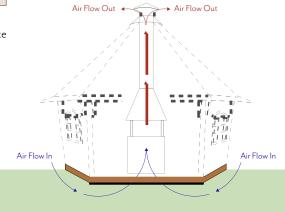
The posts allow the base frame to be slightly elevated above the ground which provides constant air flow underneath the cabin. This feeds oxygen to the BBQ unit allowing it to operate properly.
